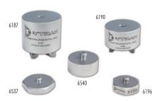
Rare earth magnets provide unsurpassed pull strength. Two pole configurations assure a steady grip on curved surfaces. Flat magnets are for use on flat surfaces for high frequency response. Use caution when applying to ferromagnetic surfaces as excessive metal to metal shock can damage unprotected accelerometers.
